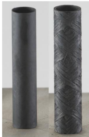
Figure 2.1 Monolithic SiC tube (left) and Triplex SiC tube (right) [11]
